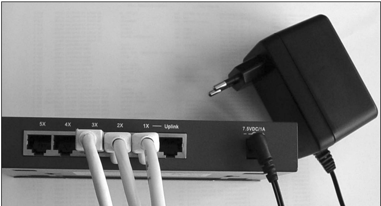
Fig. 45: Hub rear view, with the power supply and the patch cables for the three stations
