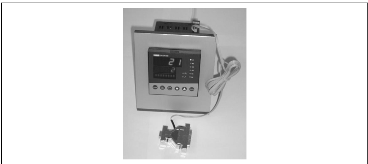
Fig. 10: Controller JUMO DICON 500 with a setup cable
