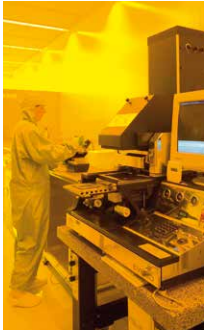
Photolithography: creating the structure on the substrate
