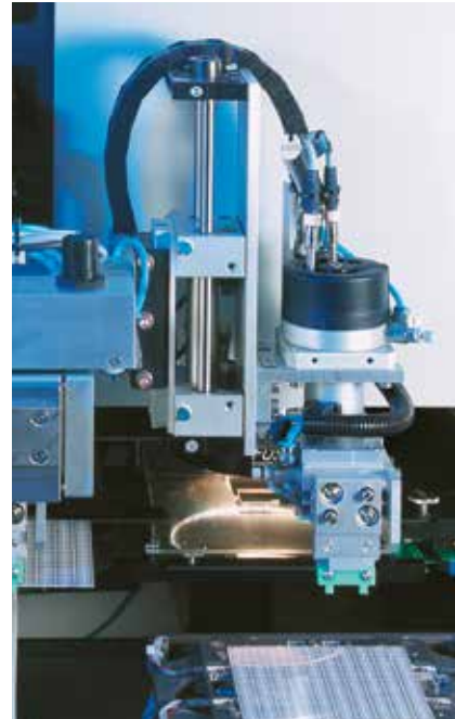
Laser trimming of platinum-chip temperature sensors
